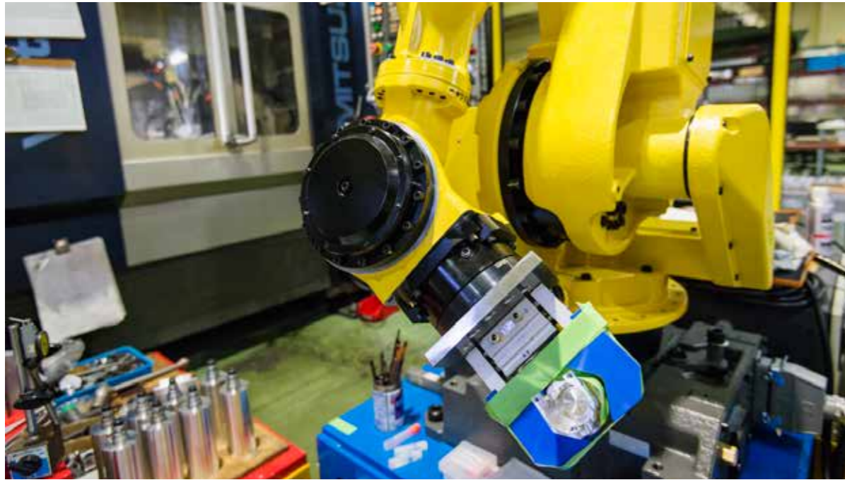
Automated production system integrating a 5-axis machining tool and a robot
